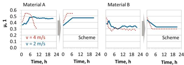
Figure 3 Cof; measured and schematic for simulation.
