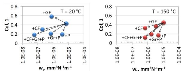
Figure 2 The effect of fillers on cof and wear  $w_s$ .
