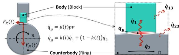
Figure 3 Basic model of the tribological system.
