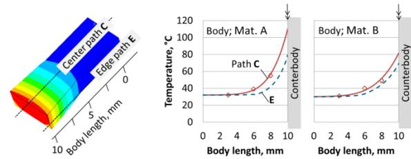
Figure 4 Temperature distributions in the body.
