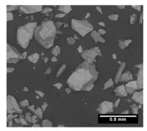
Figure 2 Close up SEM image of used garnet.
