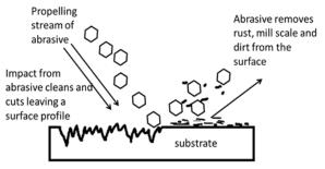
Figure 1 Mechanism of blasting process.
