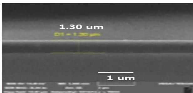
Figure 3 Cross-sectional image of ta-C coating (deposition speed was 0.6  $\mu\text{m/hr}$ , respectively).
